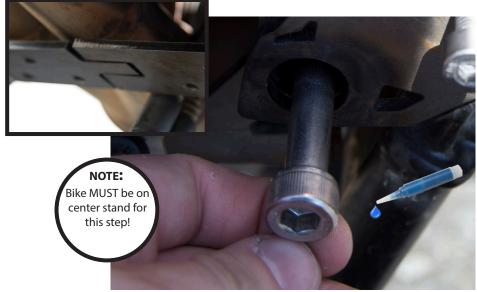
On the left side, use the T45 driver to remove large side stand bracket bolt (M10). Mount bracket, install M8 bolts, and AltRider provided M10 x 80 bolt. Do not torque anything down yet but allow them to be snug. Use thread locker. (!) Make sure that both sides of the bracket intersect properly.
