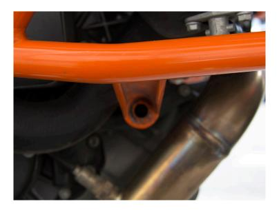
2 Remove the front M10 bolts holding the crash bars on each side.
