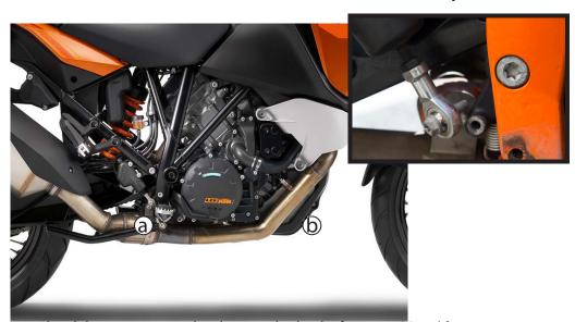
Place bike on center stand and remove both rider foot pegs (a) and foot peg mounts. To remove the right side peg, you will need to loosen the rear brake arm using a T30 driver. You will reuse all parts except for the bolts holding the peg mounts in place to the frame. Remove OEM plastic cover (b) attached to the front of the engine. TIP: If you have crash bars installed, loosen them up to make install easier.
