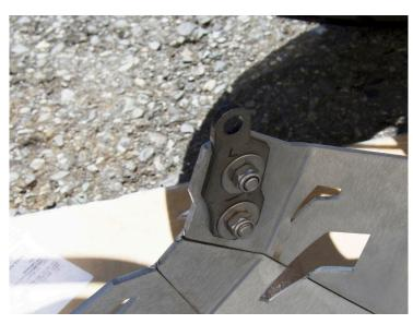
Add front brackets to the skid plate. Use the indicating marks on the brackets to place the left side bracket on the left side, facing the correct direction, triangle pointing forward. Repeat with the right side bracket. Install (4) M8 x 20 flat head bolts, washers, and nuts using a 13mm wrench and M5 allen. Snug the bolts but do not torque yet.
